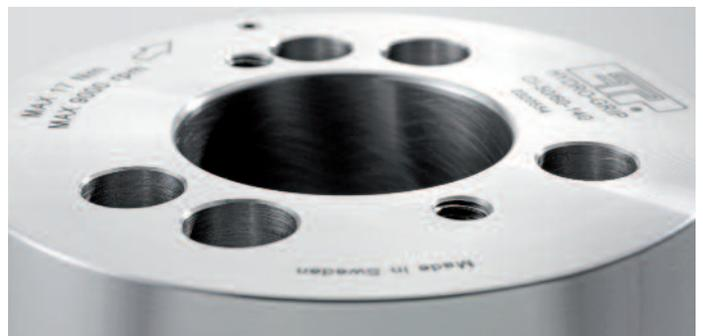
The Ø45 and Ø50 have two, threaded M8-holes for carrier pegs on a 70 mm pitch diameter. Carrier pegs, 2 pcs, 8 x 5 mm are incl.
