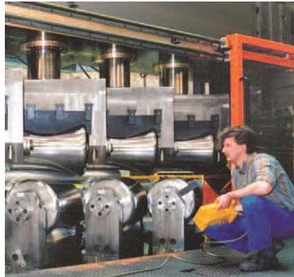
*Machine for cold forming of steel tubes. ETP-OCTOPUS locks the pistons of hydraulic cylinders, one for each cylinder, in a certain position when forming different sizes of tubes. The position is changed rather often. The locking with ETP-OCTOPUS can be done all at the same time from a central located hydraulic pump. ETP-OCTOPUS is plated in the bore with aluminium bronze to reduce wear.*
