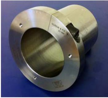
*High precision bigger size of ETP-TECHNO used in the printing industry for centering of a printing roller. The radial and also axial run out on the side of the flange has to be only some  $\mu\text{m}$ .*
