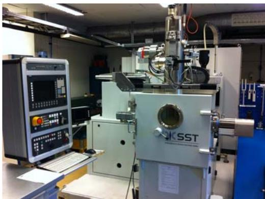
*One of our high precision electron beam welding machines.*
