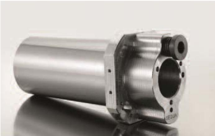
*ETP-AXPRESS with the pressure screw in the axial direction. Is designed for fastening & centering of decoration roller for printing on the outside of beverage cans. The tightening is done with a screw with a flange. The flange makes sure the screw is not overtightened. The tightening has to be in the axial direction because of the design of the machine. All unnecessary material is machined away on the flange part to reduce weight.*
