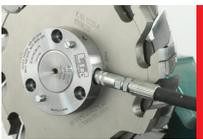
**6.** Connect the high pressure pump and increase the pressure to 400-450bar (5800-6500 psi).
