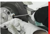
**8.** Release the pressure reduction screw on the release nipple. Remove the tool unit from the grinding machine and it is now ready to be installed on the machine.
