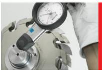
**5.** Tighten the screws (hexagon socket head, 3mm) uniformly in the locking nut. Required torque 3-4 Nm (26-35 lbf.in). Thin tools or longer sleeves (+ 120mm, 4 3/4") 6-8Nm (53-70 lbf.in)
