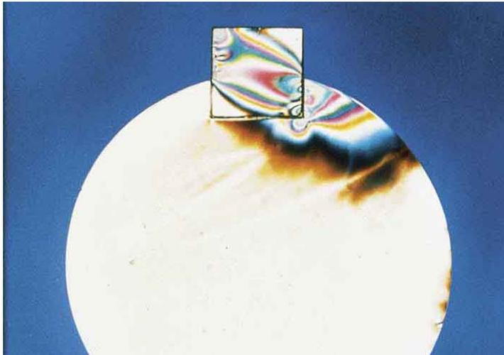
The pictures shows the stress pattern in a shaft with a keyway under pure torque.
